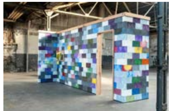
Coloured plastic bricks produced by a Precious Plastic inspired workshop
